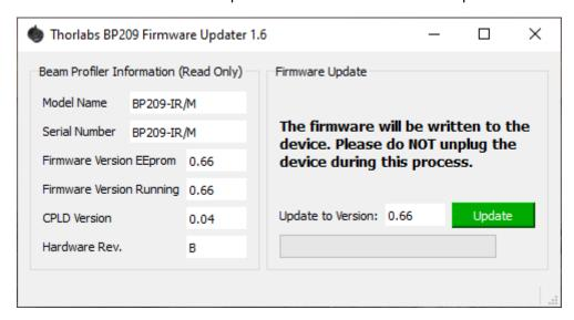
On the left side, the application shows the Beam Profiler Information. Then with pressing the "Update" Button, the update of the firmware starts. If the message "No Device Connected" is shown, the tool does not work.
